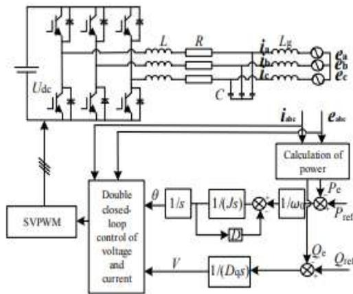
Fig.5.2 Overall block diagram of a VSG.
